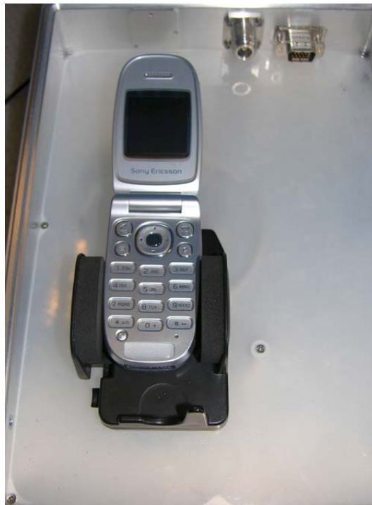
Figure 3 – Phone in Rohde & Schwartz Coupler Box
