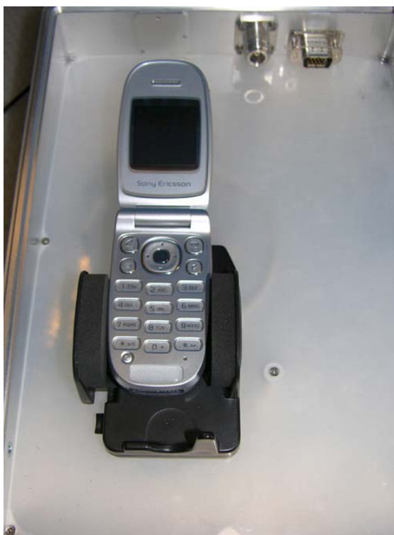
Figure 1 – Phone in Rohde & Schwartz Coupler Box
